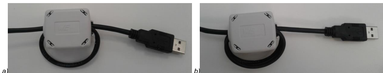
Fig. 4-21: USB cable with additional ferrite on Male-A edge with two (a) or tree (b) twists
