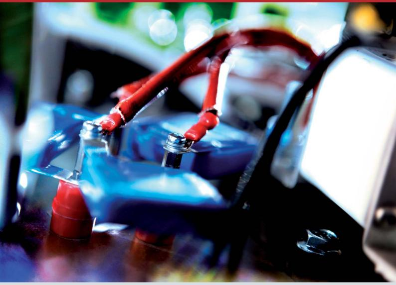
SECOMDRIVE MV IGBT Inverter are high performance water cooled drives in three level Neutral Point Clamped (NPC) topology.
