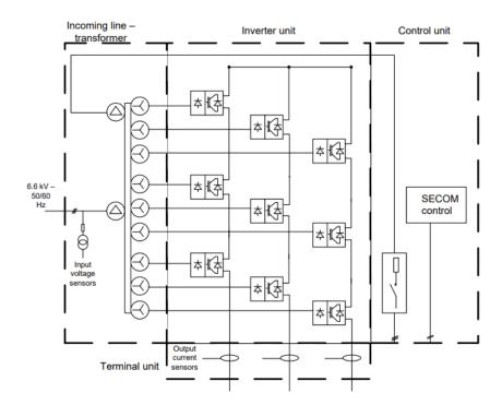
The configuration depicted in the picture above is one of the simplest that could be found and it is used to describe all the components that are always present; any other more involved configuration is always realized with the above components.
